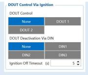
Activates a digital output when the vehicle is turned on (example: automatic flashing activation)
