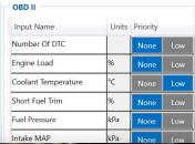
Device can be connected to ODB2 probes using bluetooth to read the vehicle's diagnostic info
