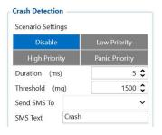
Alarm in case of an vehicle accident or crash
