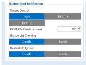
It recognizes magnetic keys and can be configured to allow ignition only if the key is correct
