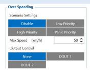
It sends an alarm or activates a digital output in case of overspeed
