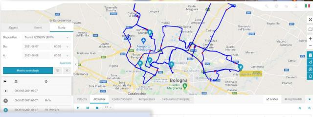
**Stored routes visualization:** vehicles position, stops details, speed and trending charts are available online on the cloud up to one year. Adding connection to the CANBUS OBD2 socket, engine information is displayed (mileage, temperature, engine rpm, fuel level, door opening, etc.)
