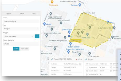
Zone management (geofence): it is possible to draw on the map areas delimited by a perimeter. Based on these, alarms can be activated in case a vehicle enters or exits, and Excel reports can be generated with the entry and exit times of all vehicles.
