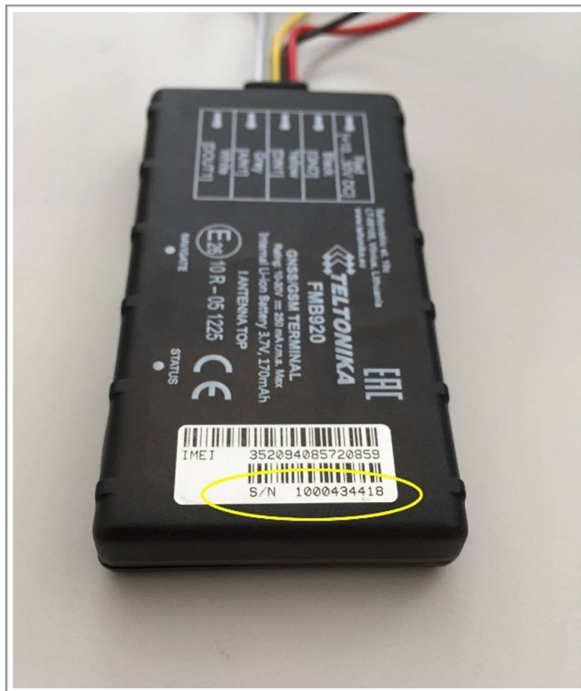
Figure 02. Identification of the tracker's IMEI code
